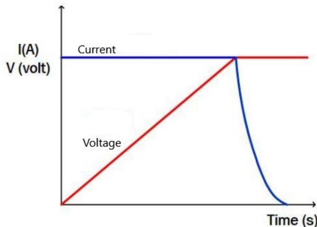
Figure 9: Constant current/constant voltage supercapacitor charge control
