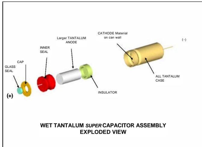
Figure 1b: AVX TWA Series Wet Tantalum Construction
