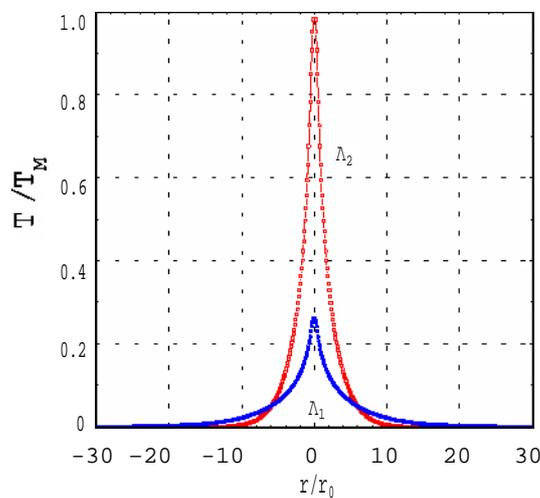
Fig.6. Normalised temperature distribution for a different thermal velocities  $\lambda_1 = 50 \text{ W/mK}$ ,  $\lambda_2 = 10 \text{ W/mK}$ .
