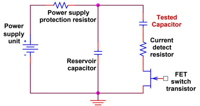
Fig.2.. Circuit of surge testing with dynamic monitoring éf features
