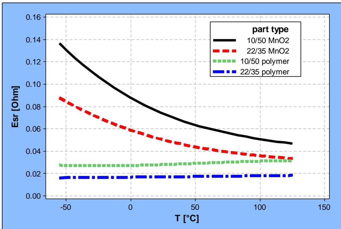
Figure 5: Temperature characteristics of ESR measured at 100kHz
