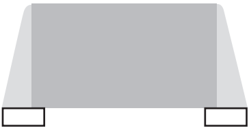
LARGE SOLDER FILLET CAN CAUSE TOMBSTONING
