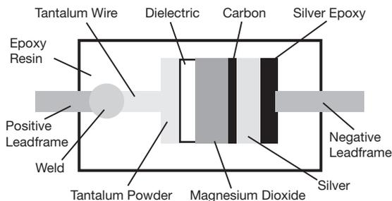
Figure 1. Stylized Surface Mount Capacitor - TAJ Range
