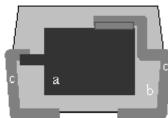
Fig.2. Tantalum capacitor construction (a – active zone, b – encapsulation case, c - leads )
