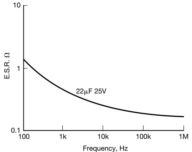
Figure 1. Typical relationship between ESR and frequency.
