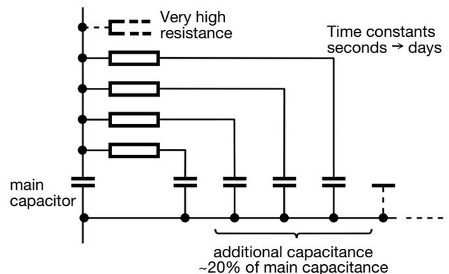
Figure 5. Dielectric absorption.
