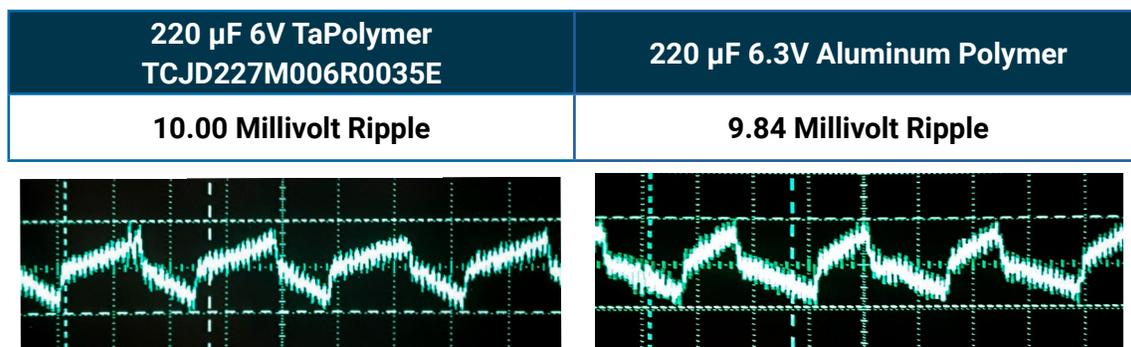
**Figure 7 Tantalum Polymer vs Aluminum Polymer Ripple Voltage**
