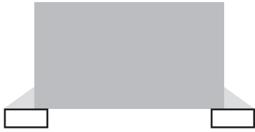
VERY SMALL FILLET WILL GIVE A POOR SOLDER YIELD
