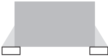
CORRECT SOLDER FILLET
