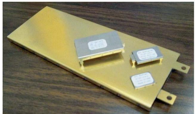
Figure 3: “Brick” BestCap® with BZ01, BZ02, and BZ05 part sizes.
