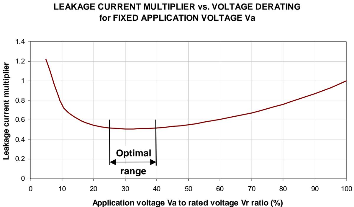
*Figure 6: Graph of maximal actual DCL vs voltage derating*
