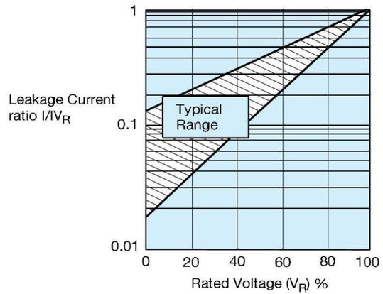
Figure 4: Effect of voltage derating on DCL
