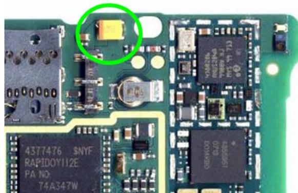
*Figure 1: Battery circuit tantalum capacitor in handheld device*
