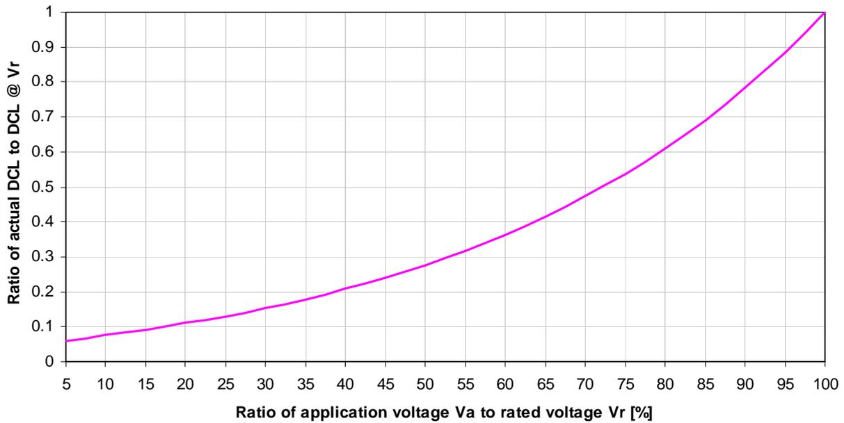
Figure 5: Median curve of typical range of DCL vs Voltage derating from Figure 4
