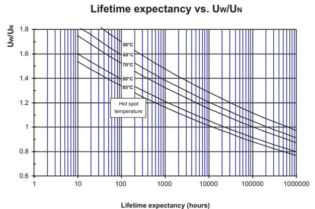
As we can see on these curves, design is done for a lifetime of 100,000 hours under the rated voltage and 70°C hot spot.
