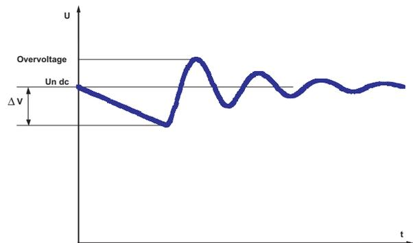
Due to the principle of carrying the power from the catenary's to the train, some contact discontinuity appears between pantograph and catenary's.
