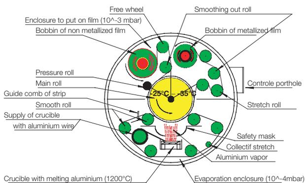
This metallized film results in the principle of self-healing which is the major reason for the increase in gradient of voltage. Even if polymer quality improves a lot, main developments are done on metallization.
