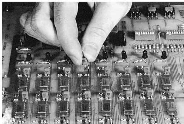
Figure 2. Inserting Capacitor on Memory Test Board
