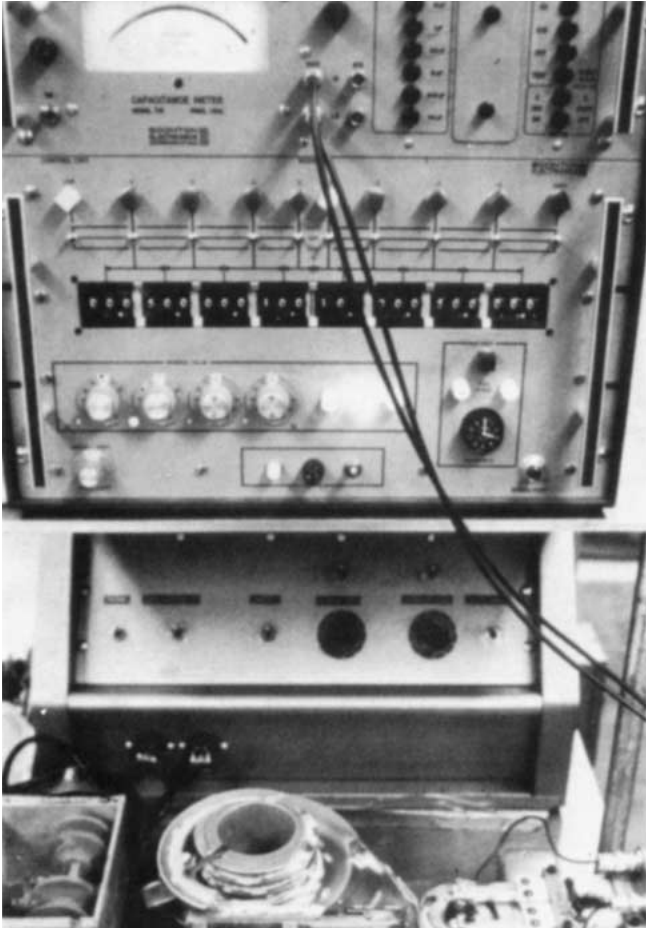
Figure 15. Testing capacitance of MLC chips
