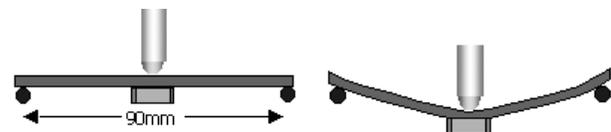
Figure 3. Board Bend Flex Test per AEC-Q200 Test Qualification
