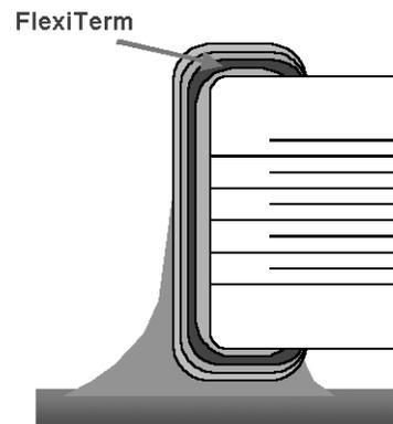
Figure 2. Additional FlexiTerm™ Layer for Increased Resistance to Mechanical Flexure
