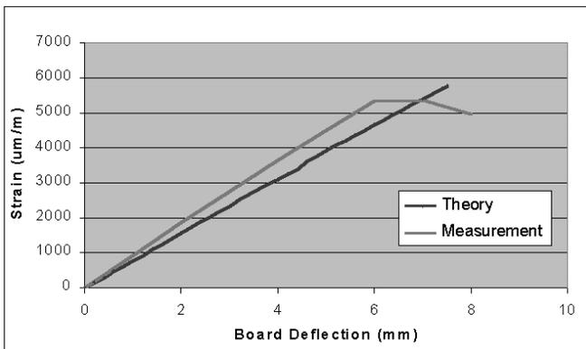
Figure 4. Calculated and Measured Strain versus Board Bend Test Deflection
