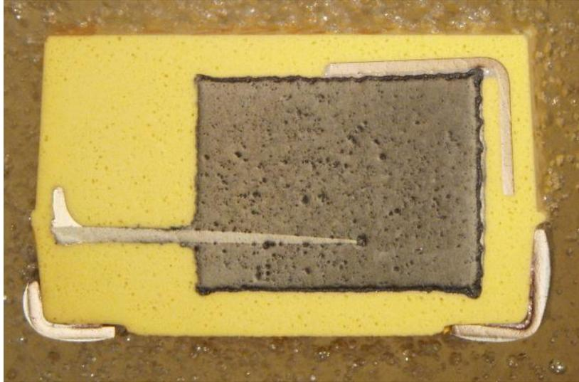
*Figure 6: Example TBJ DPA Cross Section*
