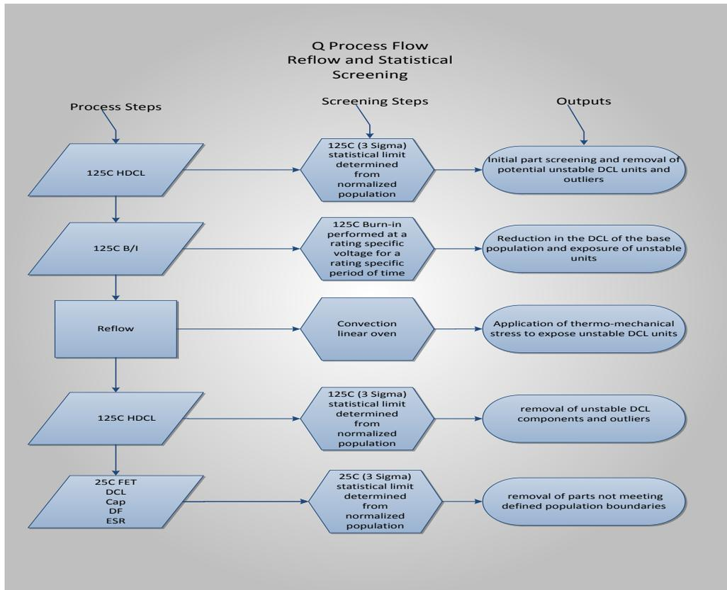
Figure 7: Q-Process Testing Flow
