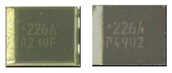
a) b) Fig. 4. New moulding compound a) pre-thermal exposure and b) post 2000 hrs at 150°C and 50 hrs at 175°C
