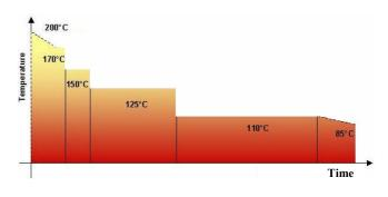
*Fig.1. Trend in time at temperature profile of tantalum capacitors*
