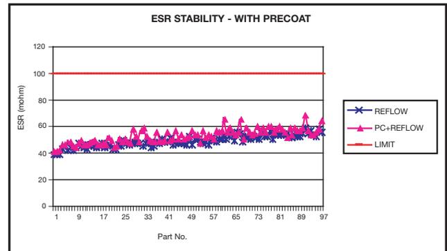
Figure 4: Effect of precoat on dielectrics
