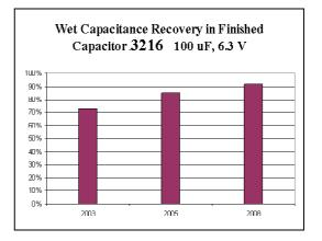
*Fig12.* Wet capacitance recovery improvement over last 5 years for case 3216, 100 μF, 6.3 V (150 kCV/g)
