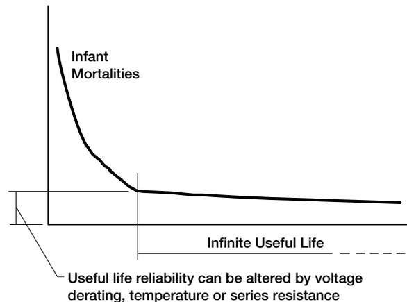
The Weibull test is a statistically monitored 40 hr burn-in – it measures the shape parameter of the curve and the final release point reliability level – and is the basis for all military and medical qualifications. For dynamic conditioning, surge test can also be applied testing either at ambient or low and high temperatures (-55°C / + 85°C).
