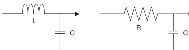
Initial investigations were done using either ferrite beads having 33 ohms and 120 ohms of impedance at 100 MHz. Resistors of 33 ohms and 100 ohms resistance were used in the R-C investigation.
