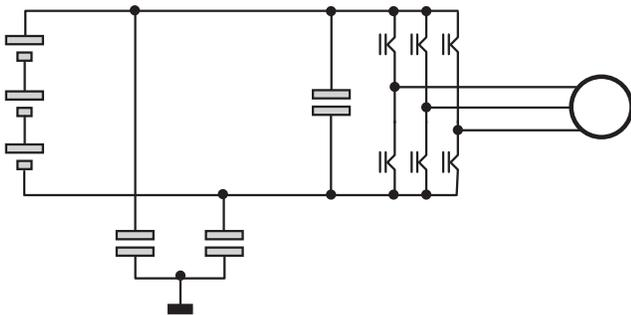
In that case, capacitor will be used as a decoupling capacitor. Film capacitor is particularly well adapted for this use, because main criteria for DC link capacitor will be rms. current withstanding.
