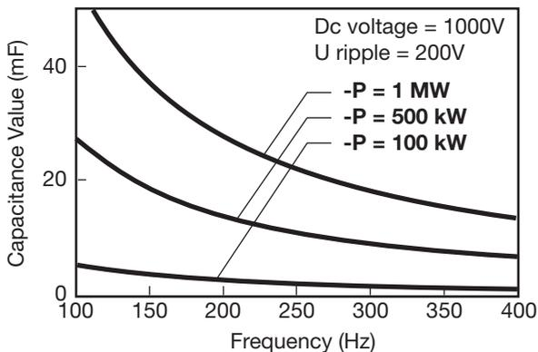
To compare with electrolytic solution, we will take a current capability of 20mA per  $\mu\text{F}$  for electrolytic capacitors. First case, power at 1Mwatt:
