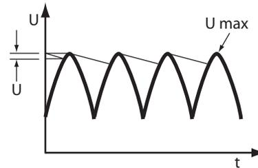
Capacitance value will be defined taken in account that supply frequency is lower than converter frequency.
