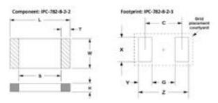
IPC has set a standard of recommended footprints for most classes of surface mount electronic components including resistors, capacitors and inductors.
