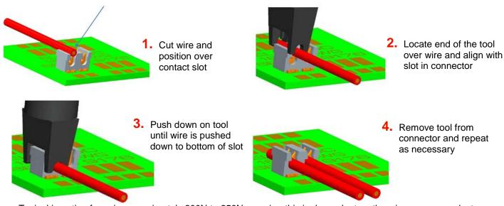
Typical insertion force is approximately 200N to 250N per wire, this is dependent on the wire gauge, conductor strands and insulation material.
