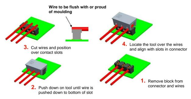
Typical insertion force is 250N to 350N per wire, this is dependent on the wire gauge, number of conductor strands and insulation material.
