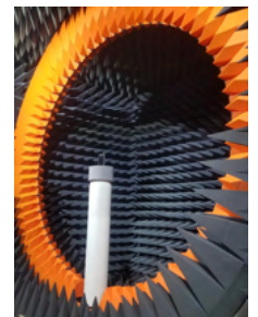
Anechoic Chamber 400 MHz - 18 GHz
